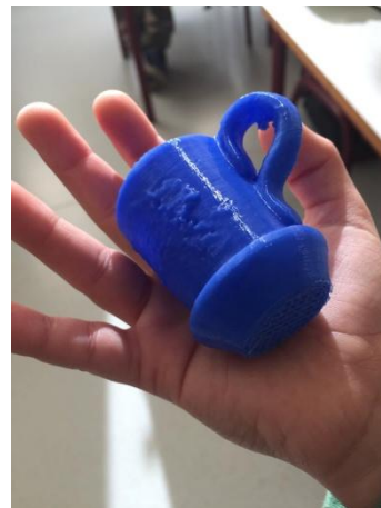
3D printed workpiece of intangible local heritage (Bajouca pottery) scanned with Creality
